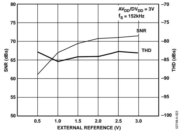
Figure 16. Typical Dynamic Performance vs.  $V_{REF}$ ,  $V_{DD} = 3 V$
