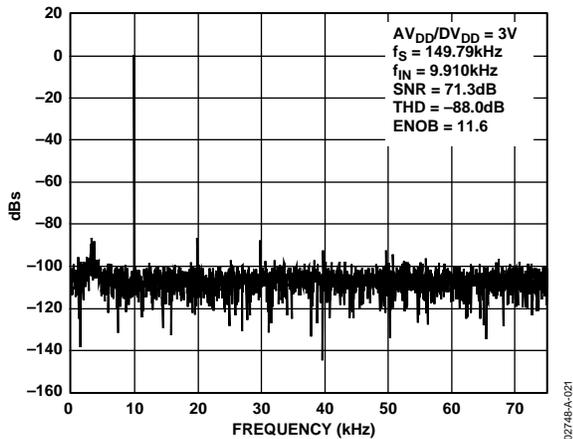
Figure 14. ADuC814 Dynamic Performance at  $V_{DD} = 3 V$
