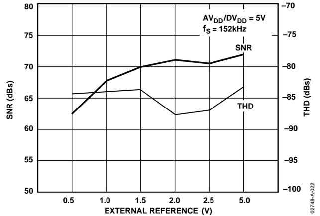
Figure 15. Typical Dynamic Performance vs.  $V_{REF}$ ,  $V_{DD} = 5 V$
