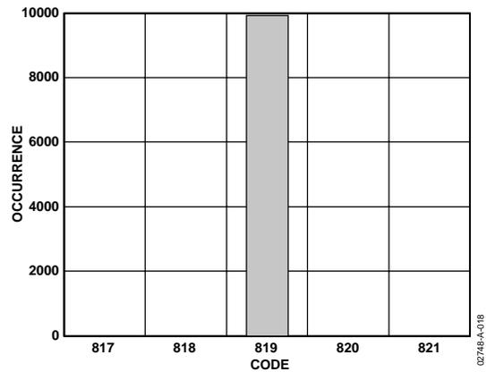
Figure 11. Code Histogram plot,  $V_{DD} = 5\text{ V}$
