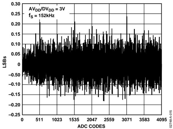
Figure 8. Typical DNL Error,  $V_{DD} = 3\text{ V}$
