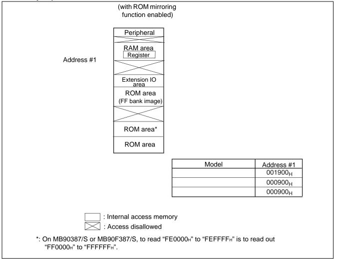
Note: When internal ROM is operating, F<sup>2</sup>MC-16LX allows viewing ROM data image on FF bank at upper-level of 00 bank. This function is called "mirroring ROM," which allows effective use of C compiler small model.
