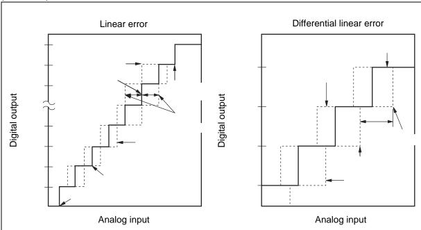
$$Linear\ error\ of\ digital\ output\ N = \frac{V_{NT} - \{1\ LSB \times\ (N-1) + V_{OT}\}}{1\ LSB} [LSB]$$
