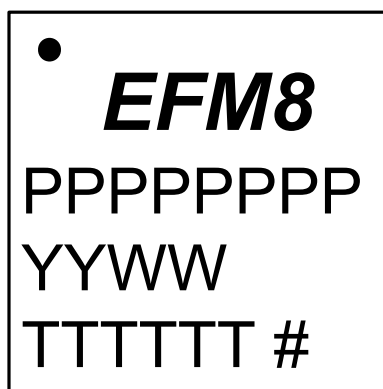
Figure 7.3. QFN32 Package Marking
