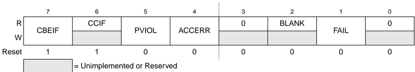
**Figure 27-13. Flash Status Register (FSTAT — Special Mode)**
