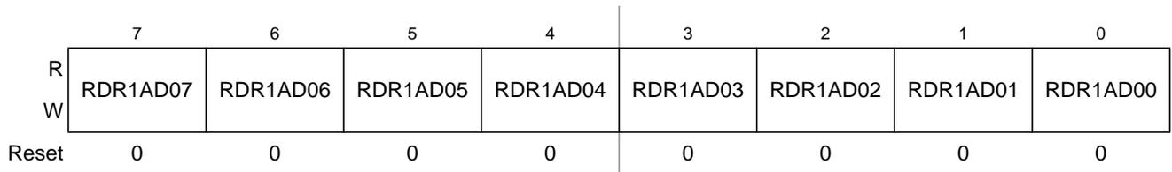
Figure 22-66. Port AD0 Reduced Drive Register 1 (RDR1AD0)
