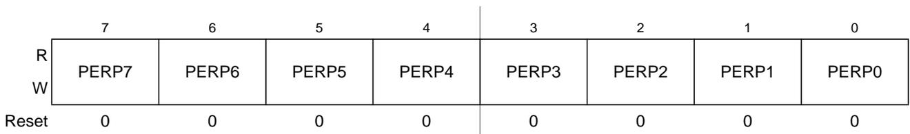
Figure 22-44. Port P Pull Device Enable Register (PERP)
