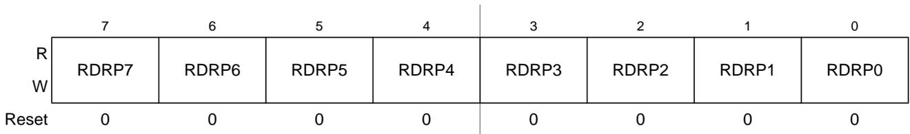
Figure 22-43. Port P Reduced Drive Register (RDRP)
