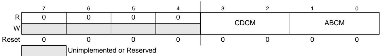
**Figure 19-6. Debug Control Register2 (DBGC2)**
