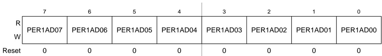
Figure 22-67. Port AD0 Pull Up Enable Register 1 (PER1AD0)
