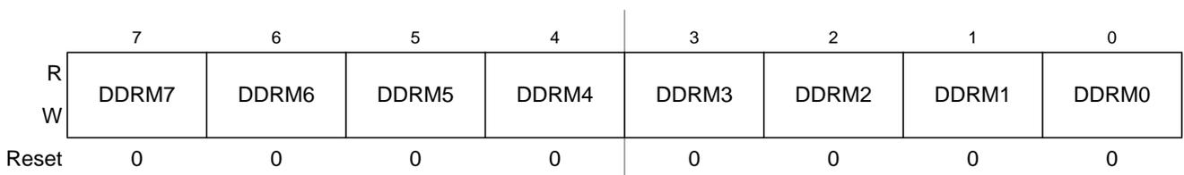
**Figure 24-30. Port M Data Direction Register (DDRM)**
