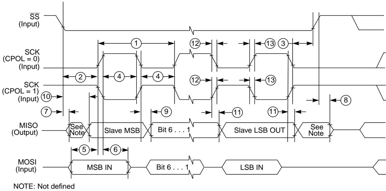
**Figure A-9. SPI Slave Timing (CPHA = 0)**
