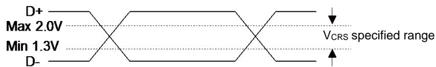
\*5: They indicate rise time ( $T_{RISE}$ ) and fall time ( $T_{FALL}$ ) of the full-speed differential data signal.
