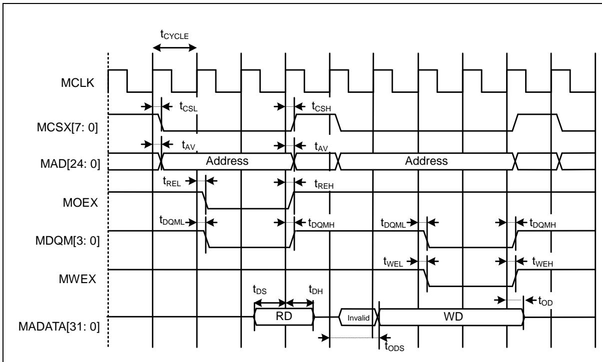
**When Using Synchronous Serial Chip Select (SCINV = 1, CSLVL = 0)**
