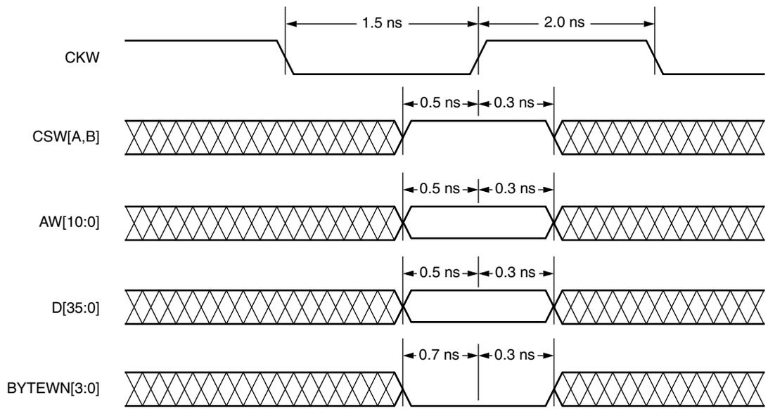
**Figure 36. Minimum Timing Specs for Memory Blocks-Read Cycle (-1 Speed Grade)**
