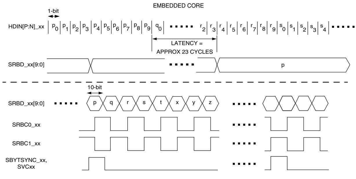
With the 8b10bR\_xx control bit of the SERDES channel set to 1, the data presented at SRBD\_xx[9:0] will be decoded characters. Bit 8 will indicate whether SRBDxx[7:0] represents an ordinary data character (bit 8 = 0), or whether SRBD\_xx[7:0] represents a special character, like a comma. Bit 9 may be either a code violation indicator or one of seven out of synchronization state indicators, as described later.
