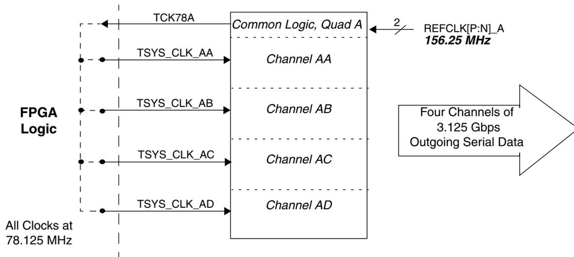
If the transmit line rate is mixed between half and full rate among the channels, then the scheme shown in Figure 26 can be used. The figure shows TSYS\_CLK\_AA and TSYS\_CLK\_AB being sourced by TCK78A and TSYS\_CLK\_AC and TSYS\_CLK\_AD being sourced by TCK78A/2 (the division is done in FPGA logic). Similar clocking would be used for Quad B.
