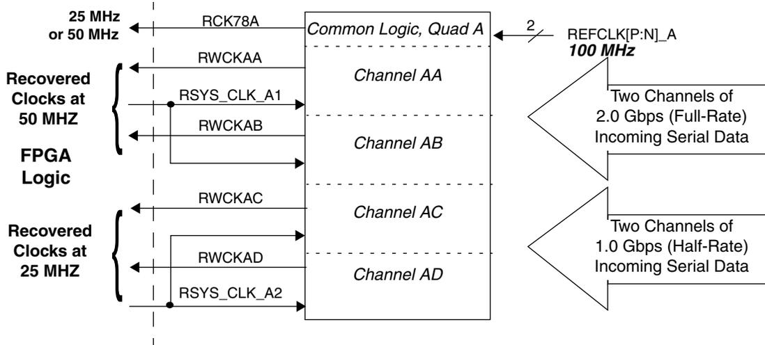
As noted in the caption of Figure 28, each quad can be configured in any line rate (0.6 to 3.7 Gbps), since each quad has its own reference clock input pins. The receive alignment FIFO per channel cannot be used in this mode.
