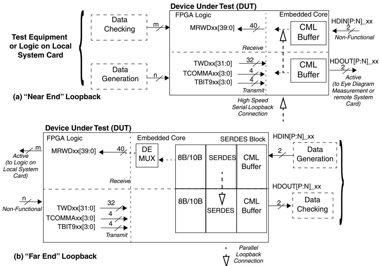
The loopback mode can also be characterized by the physical location of the loopback connection. There are three possible loopback modes supported by the Embedded Core logic:
