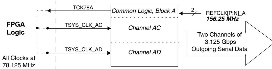
If the transmit line rate is mixed between half and full rate among the channels, then the scheme shown in Figure 19 can be used. The figure shows TSYS\_CLK\_AC being sourced by TCK78A and TSYS\_CLK\_AD being sourced by TCK78A/2 (the division is done in FPGA logic). Similar clocking would be used for Block B.
