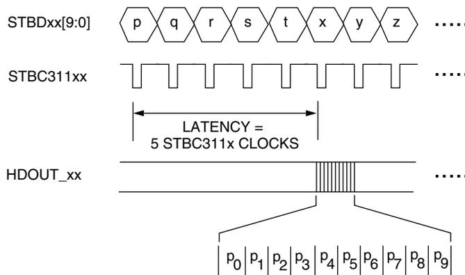
Each block also sends a clock to the FPGA logic. This clock, TCK78[A,B], is sourced from one of the four MUX blocks and has the same frequency as TSYS\_CLK\_xx, but arbitrary phase. Within each MUX block, the low frequency clock output is obtained by dividing by 4 the SERDES STBC311x clock which is used internally to synchronize the transmit data words. TCKSEL control bits select the channel to source TCK78[A:B].
