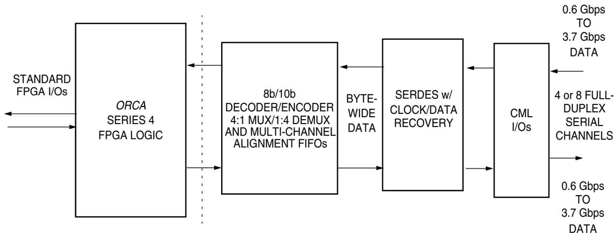
The serial channels can each operate at up to 3.7 Gbps (2.96 Gbps data rate) with a full-duplex synchronous interface with built-in clock recovery (CDR). The 8b/10b encoding provides guaranteed ones density for the CDR, byte alignment, and error detection. The core is also capable of frame synchronization and physical link monitoring and contains independent 4k x 36 RAM blocks. Overviews of the various blocks in the embedded core are presented in the following paragraphs.
