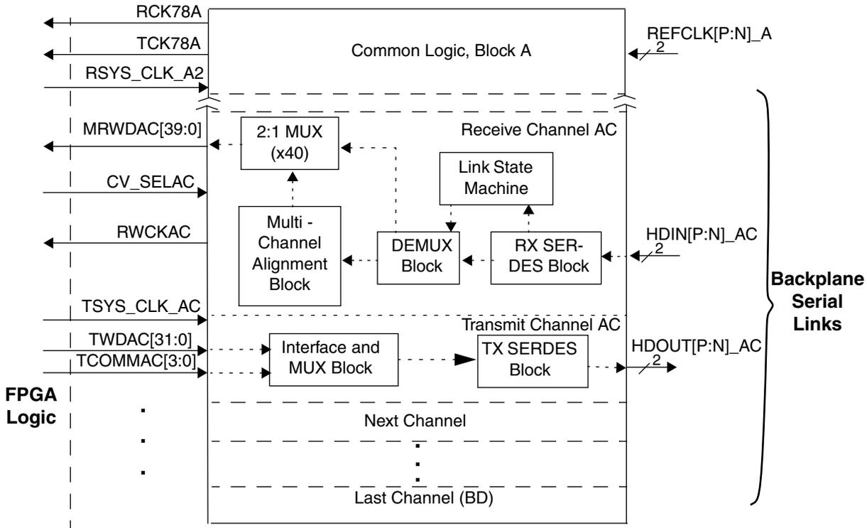
The Embedded Core provides transceiver functionality for four or eight serial data channels and is organized into two blocks, each supporting two or four channels. Each channel is identified by both a block identifier [A:B] and a channel identifier [A:D]. In the ORT42G5 only the channel identifiers C and D are used. (This naming convention follows that of the ORT82G5).
