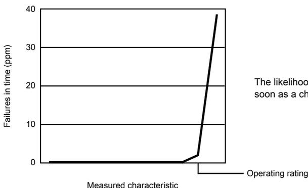
The likelihood of permanent chip failure increases rapidly as soon as a characteristic begins to exceed one of its operating ratings.
