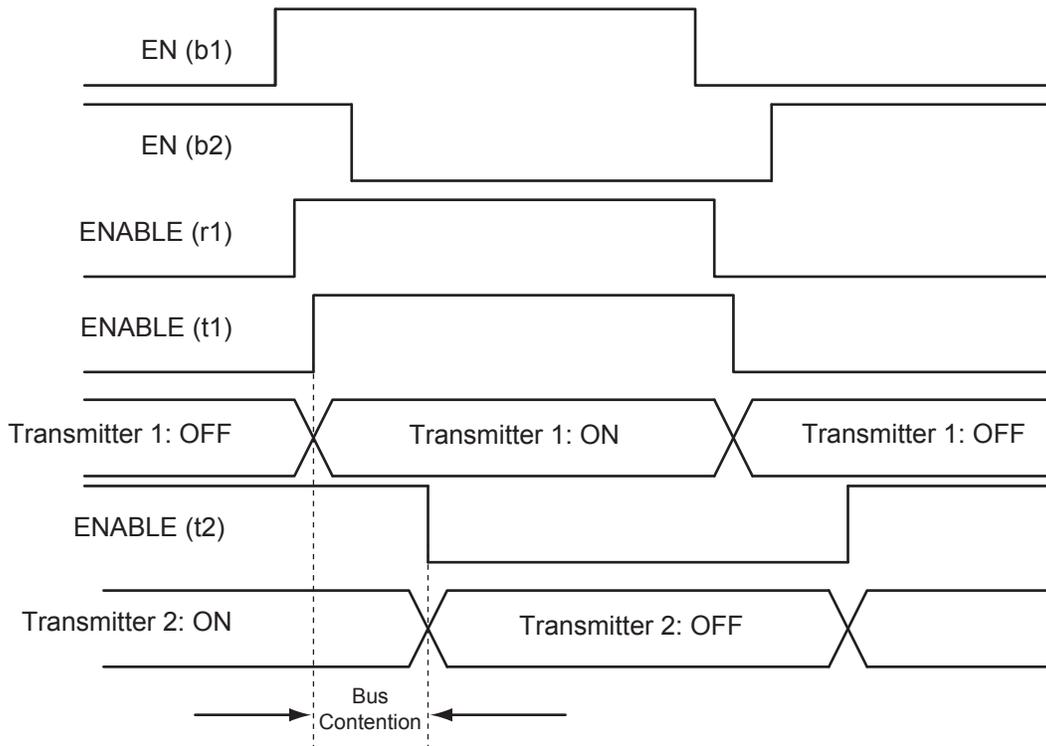
**Figure 2-111 • Timing Diagram (bypasses skew circuit)**
