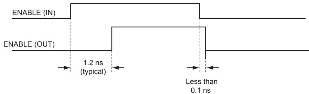
**Figure 2-109 • Timing Diagram (option 2: enables skew circuit)**
