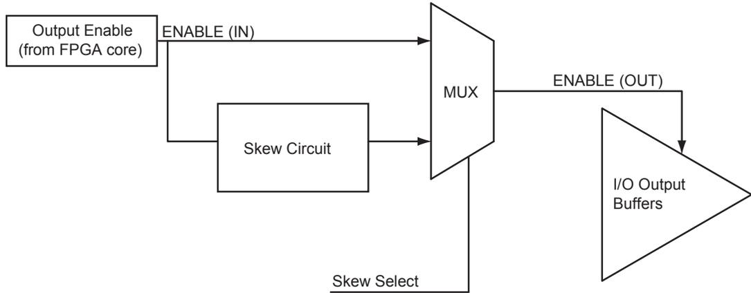
**Figure 2-107 • Block Diagram of Output Enable Path**
