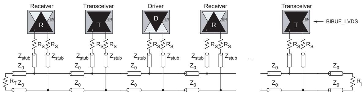
**Figure 2-135 • BLVDS/M-LVDS Multipoint Application Using LVDS I/O Buffers**
