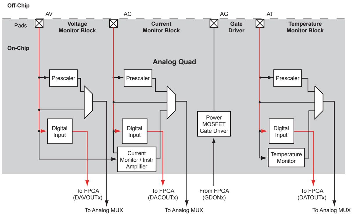
**Figure 2-69 • Analog Quad Direct Digital Input Configuration**
