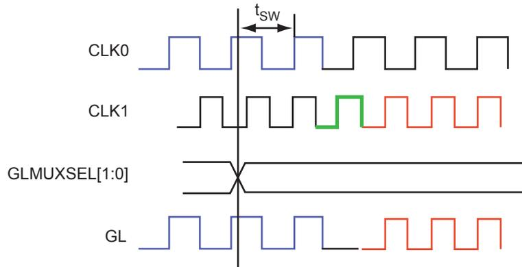
**Figure 2-26 • NGMUX Waveform**
