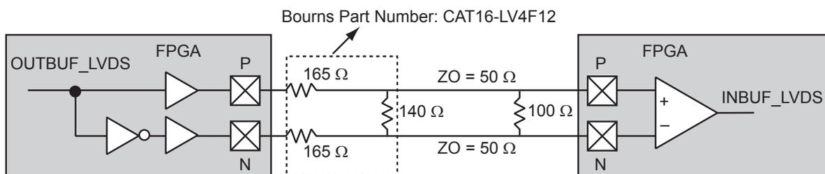
**Figure 2-134 • LVDS Circuit Diagram and Board-Level Implementation**
