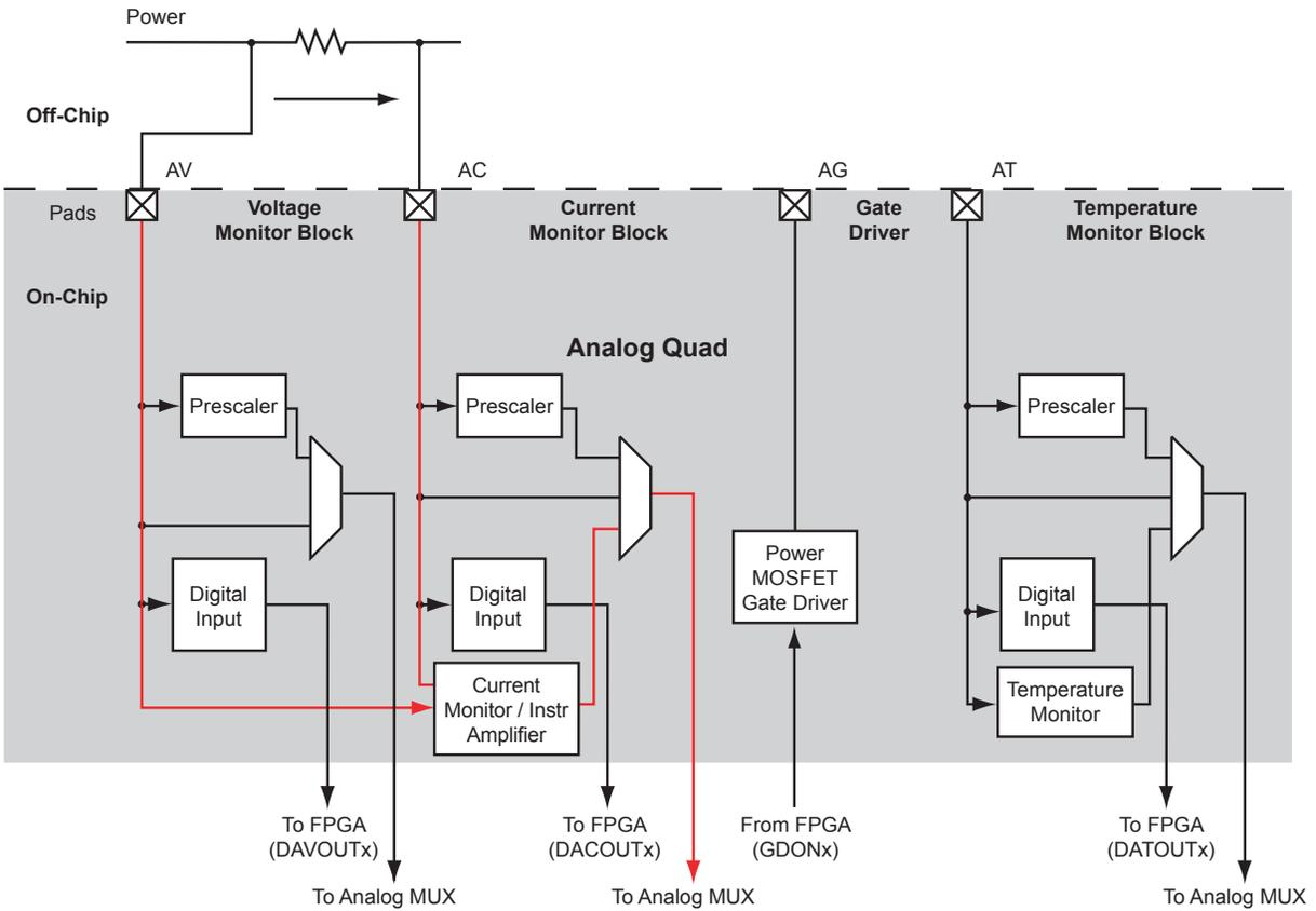
**Figure 2-70 • Analog Quad Current Monitor Configuration**
