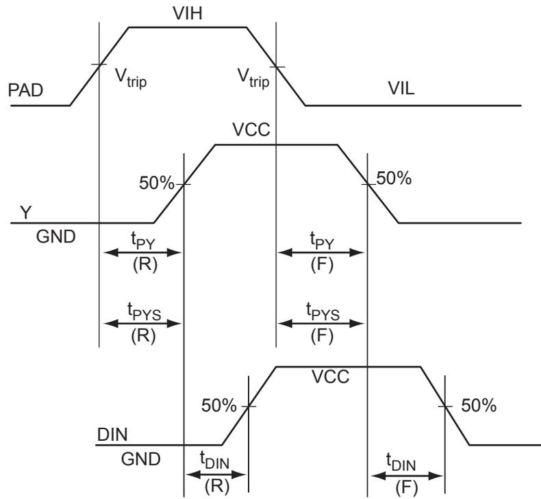
**Figure 2-116 • Input Buffer Timing Model and Delays (example)**
