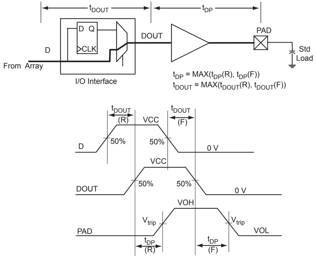
Figure 2-117 • Output Buffer Model and Delays (example)
