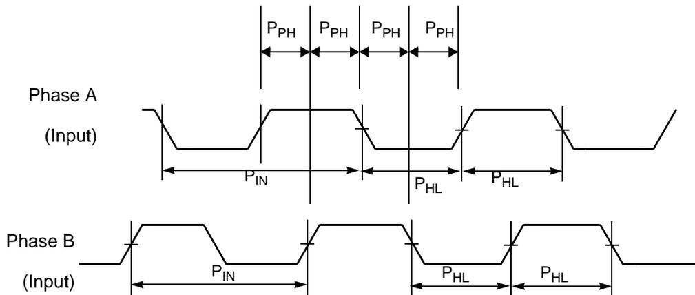
**Figure 3-24 Quadrature Decoder Timing**
