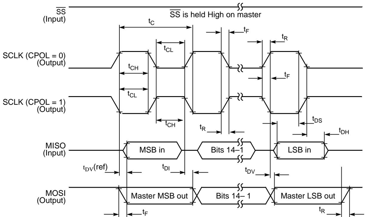
**Figure 3-20 SPI Master Timing (CPHA = 1)**
