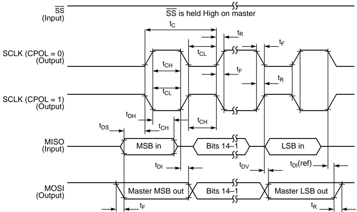
**Figure 3-19 SPI Master Timing (CPHA = 0)**
