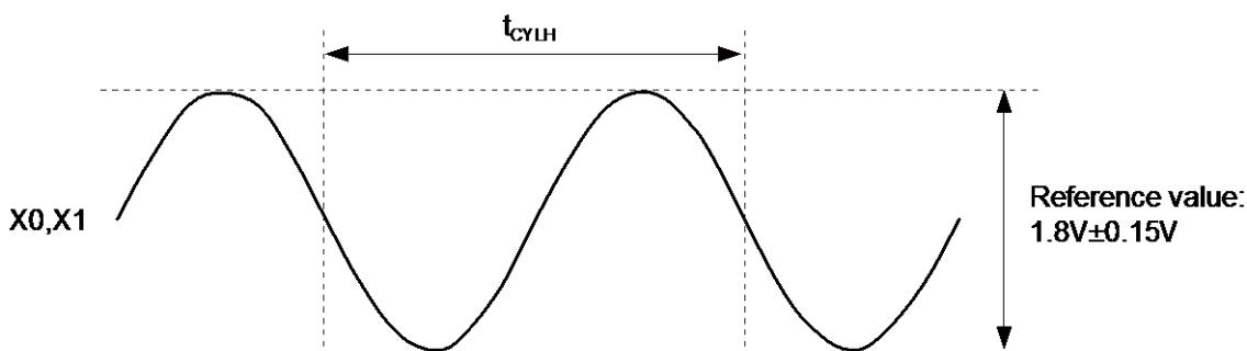
The amplitude changes by resistance, capacity which added outside or the difference of the device.
