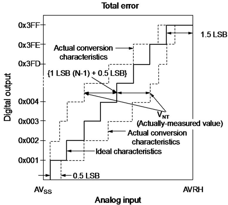
$$1\text{LSB (Ideal value)} = \frac{\text{AVRH} - \text{AV}_{\text{SS}}}{1024} \text{ [V]}$$
