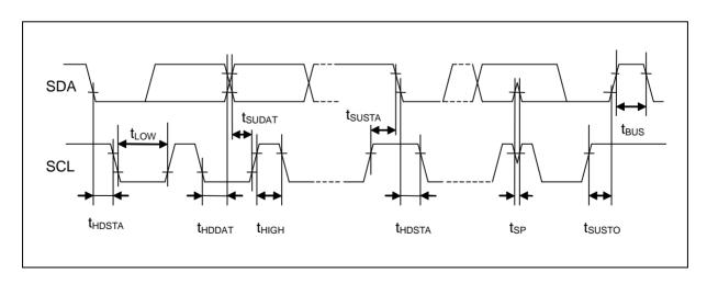
$<sup>^{\</sup>star 2}$ : The maximum  $t_{HDDAT}$  only has to be met if the device does not extend the "L" width  $(t_{LOW})$  of the SCL signal.
