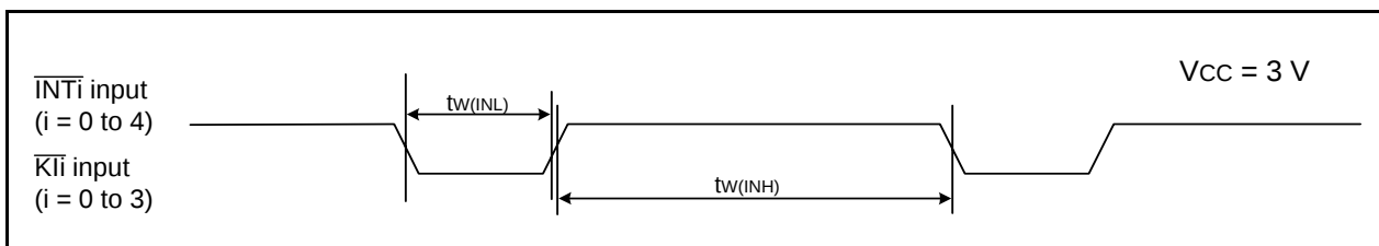
Figure 5.15 Input Timing Diagram for External Interrupt \overline{INTi} and Key Input Interrupt \overline{Kli} when Vcc = 3 V
