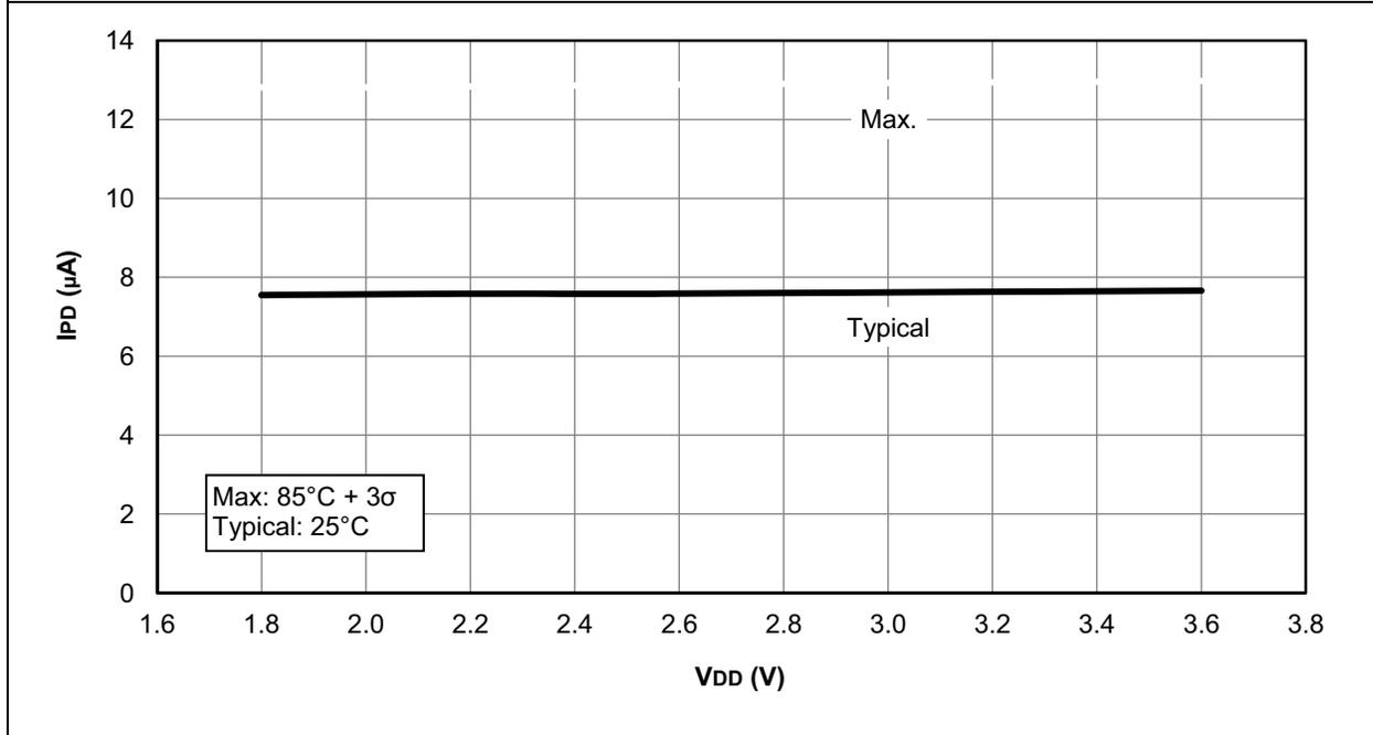
**FIGURE 29-32: I<sub>PD</sub>, COMPARATOR, LOW-POWER MODE (C<sub>x</sub>SP = 0), PIC16F1503 ONLY**
