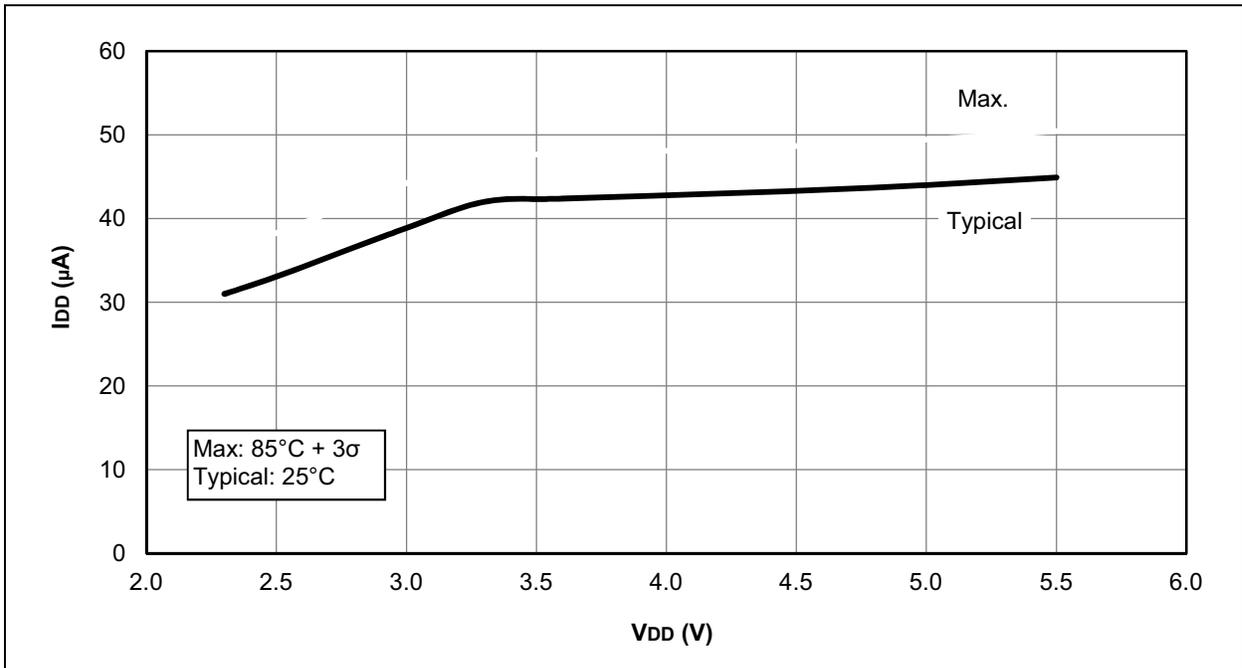
**FIGURE 29-31: I<sub>PD</sub>, COMPARATOR, LOW-POWER MODE (C<sub>x</sub>SP = 0), PIC16LF1503 ONLY**
