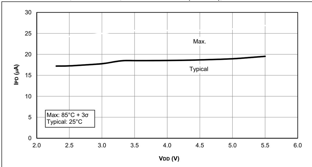
**FIGURE 29-43: BROWN-OUT RESET VOLTAGE, BORV = 1, PIC16LF1503 ONLY**
