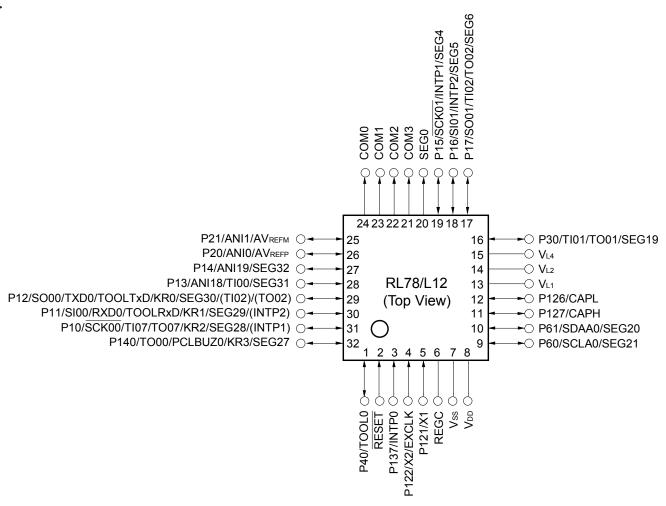
Caution Connect the REGC pin to Vss via a capacitor (0.47 to 1  $\mu$ F).
