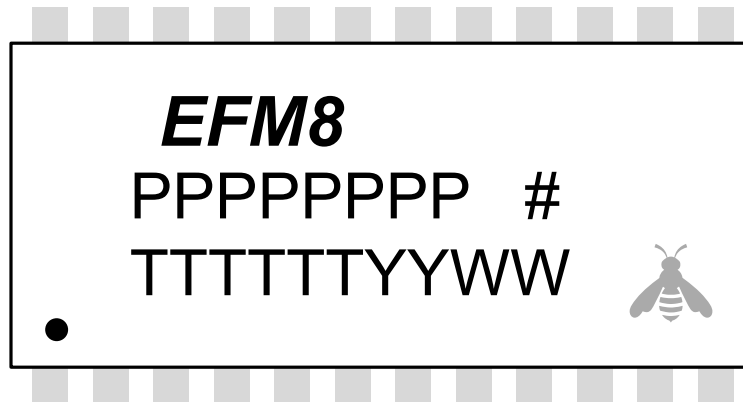
Figure 10.3. QSOP24 Package Marking
