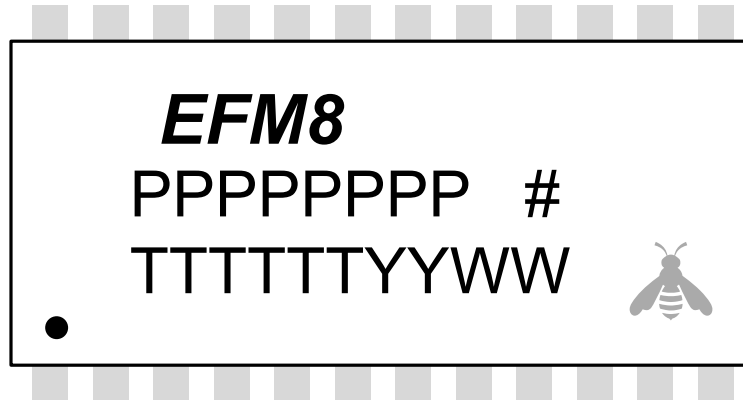
Figure 10.3. QSOP24 Package Marking
