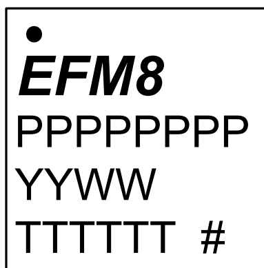
Figure 7.3. QFN32 Package Marking
