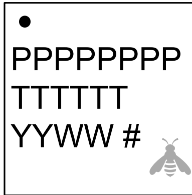
Figure 8.3. QFN24 Package Marking
