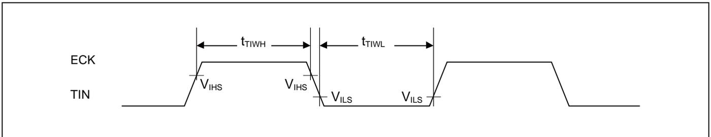
**Trigger input timing**
