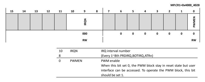
Basically, PRDIRQ and BOTIRQ are generated every period. However, the interrupt interval can be controlled from 0 to 8 periods. When IRQN.CR1 = 0, the interrupt is requested every period, otherwise the interrupt is requested every (IRQN+1) times of period.
