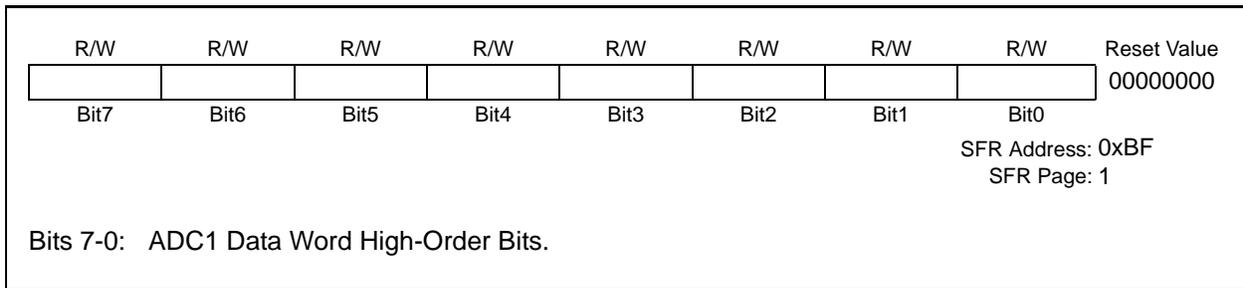
**Figure 5.17. ADC1L: ADC1 Data Word LSB Register**
