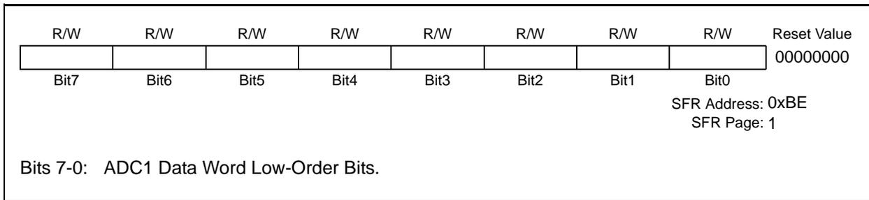
**Figure 5.18. ADC1 Data Word Example**
