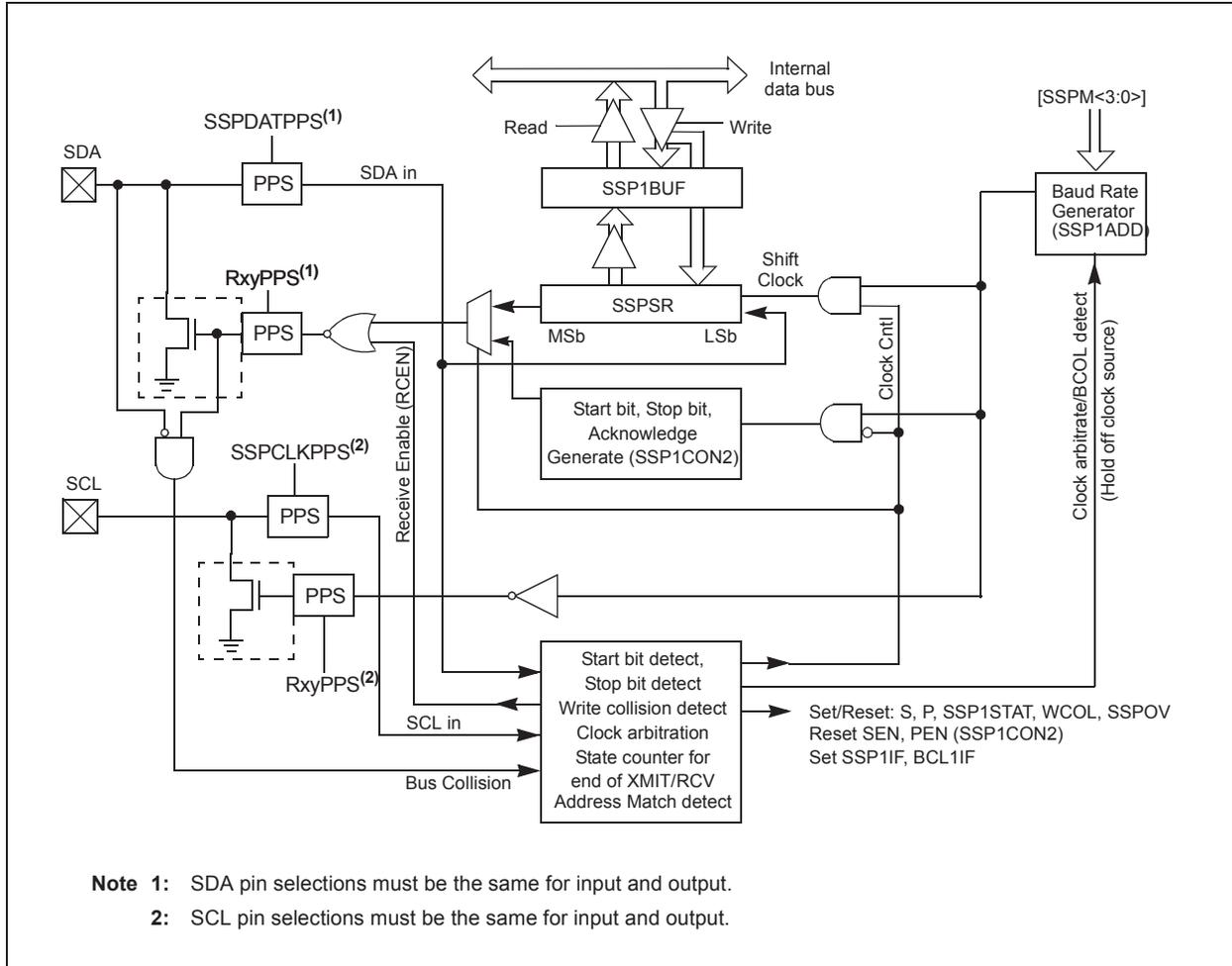
FIGURE 32-14: I<sup>2</sup>C SLAVE, 7-BIT ADDRESS, RECEPTION (SEN = 0, AHEN = 0, DHEN = 0)
