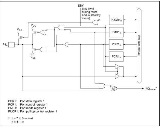
Figure C.1 (a) Port 1 Block Diagram (Pins P1<sub>7</sub> to P1<sub>4</sub>)
