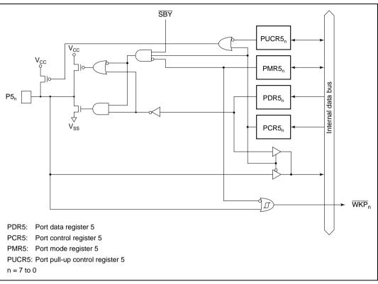
Figure C.4 Port 5 Block Diagram
