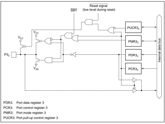
Figure C.2 (e-3) Port 3 Block Diagram (Pin P3<sub>2</sub> in the F-ZTAT Version of the H8/38327 Group and H8/38427 Group)
