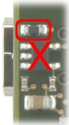
Figure 9: assembly option for VCCAUX = 3.3 V (bottom view).
