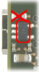
Figure 8: assembly option for VCCAUX = 2.5 V (bottom view).
