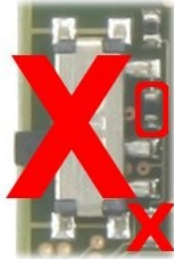
Figure 38: Assembly option: S2 = FX2 PON.
