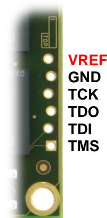
Figure 24: JTAG connector J2.
