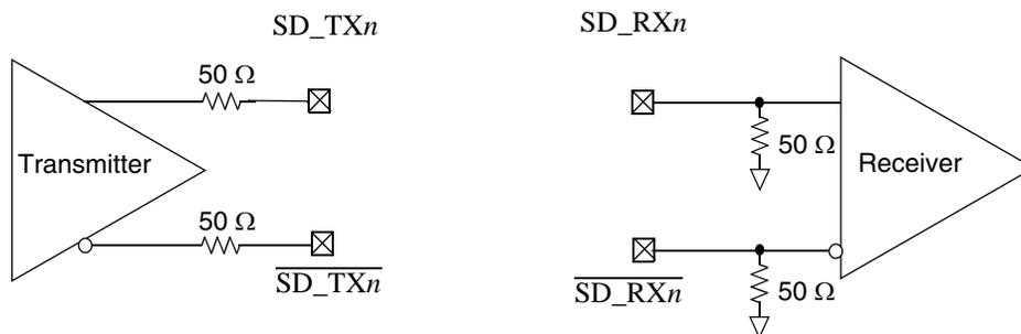
Figure 39. SerDes Transmitter and Receiver Reference Circuits
