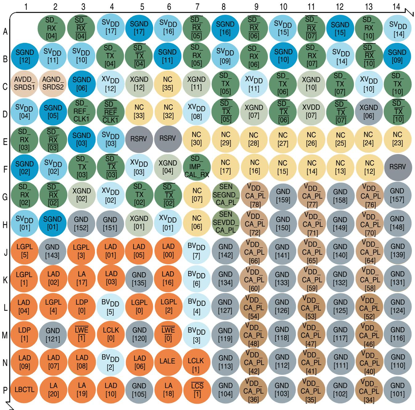
Figure 3. 780 BGA Ball Map Diagram (Detail View A)
