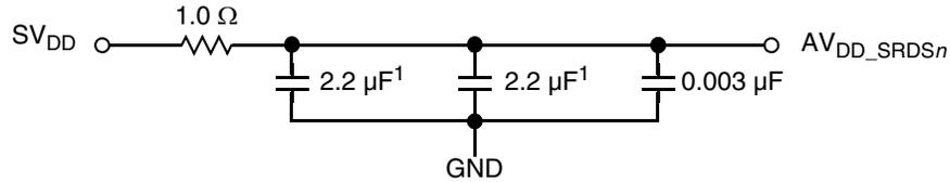
Figure 51. SerDes PLL Power Supply Filter Circuit
