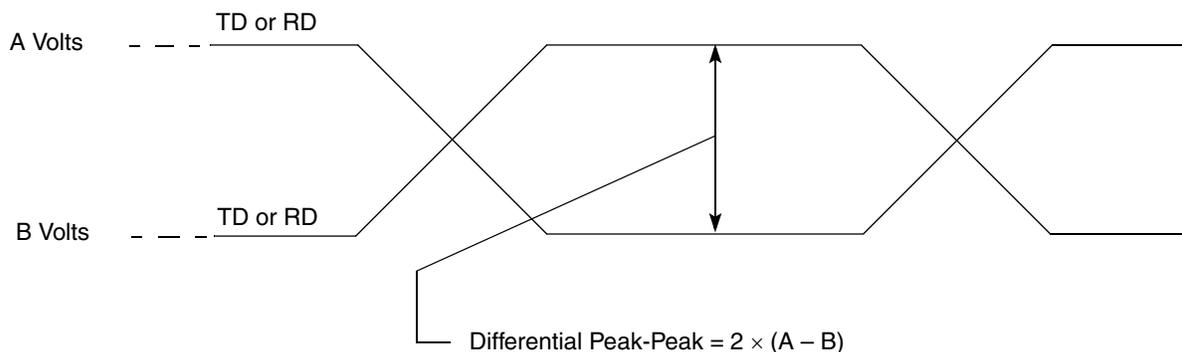
**Figure 41. Differential Peak-Peak Voltage of Transmitter or Receiver**
