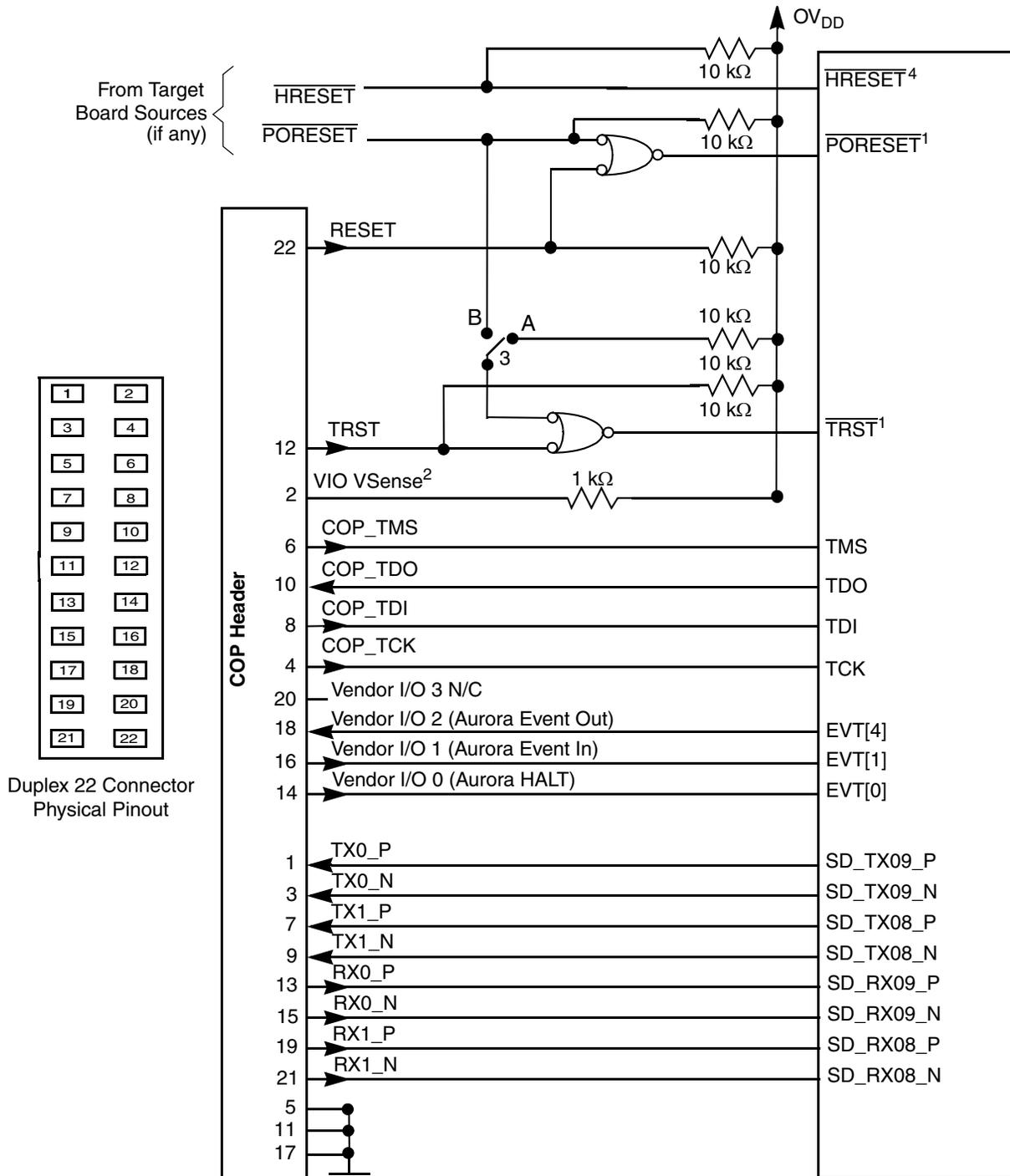
Figure 58. Aurora 22 Pin Connector Duplex Interface Connection
