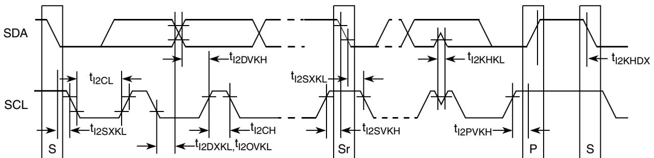
Figure 30. I<sup>2</sup>C Bus AC Timing Diagram
