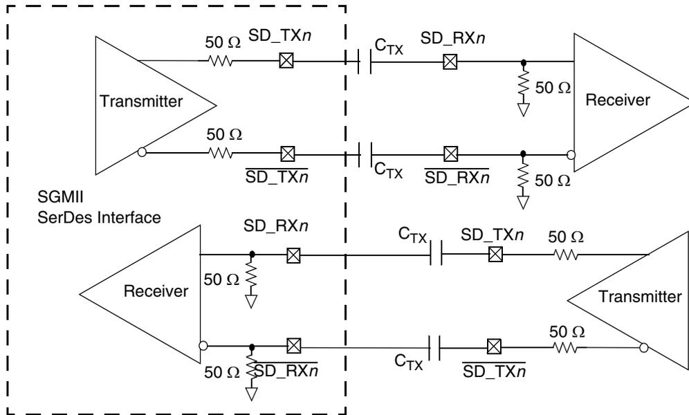
**Figure 44. 4-Wire AC-Coupled SGMII Serial Link Connection Example**
