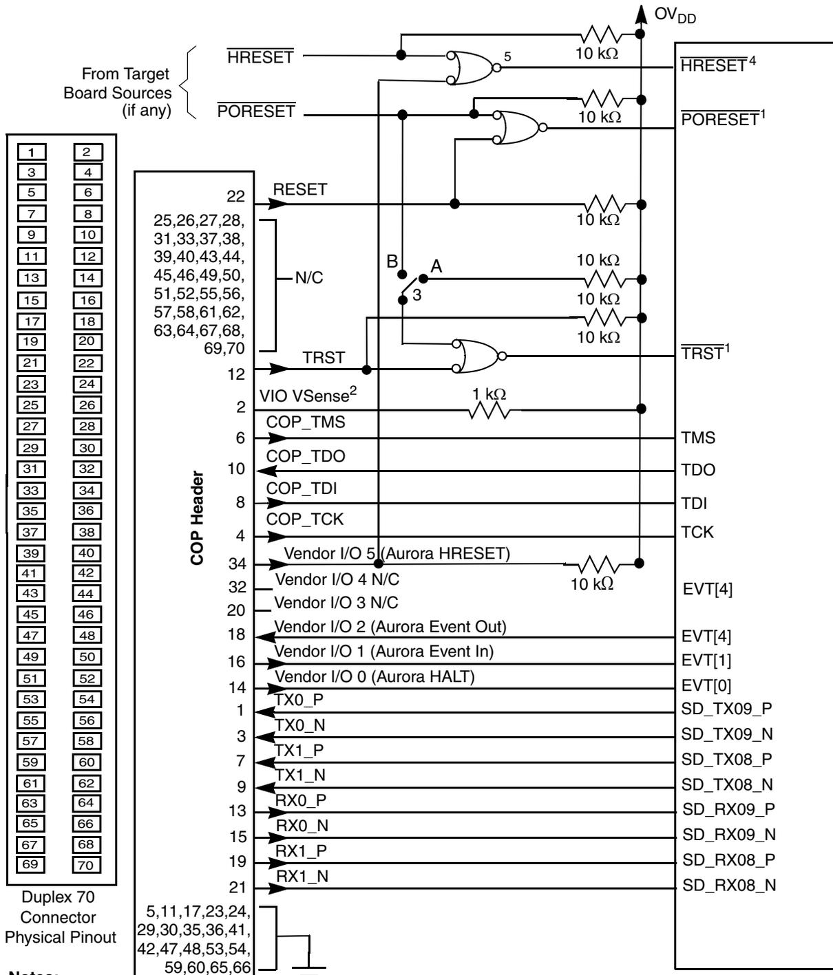
Figure 59. Aurora 70 Pin Connector Duplex Interface Connection
