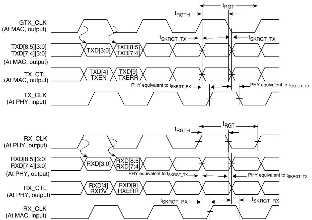
Figure 16. RGMII AC Timing and Multiplexing Diagrams
