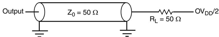
**Figure 25. AC Test Load for the JTAG Interface**
