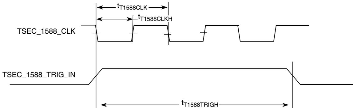
**Figure 19. eTSEC IEEE 1588 Input AC Timing**
