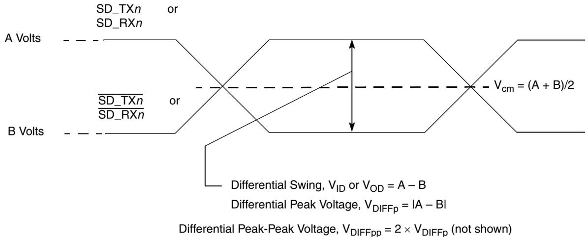
**Figure 32. Differential Voltage Definitions for Transmitter or Receiver**
