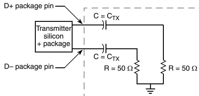
**Figure 40. Test/Measurement Load**
