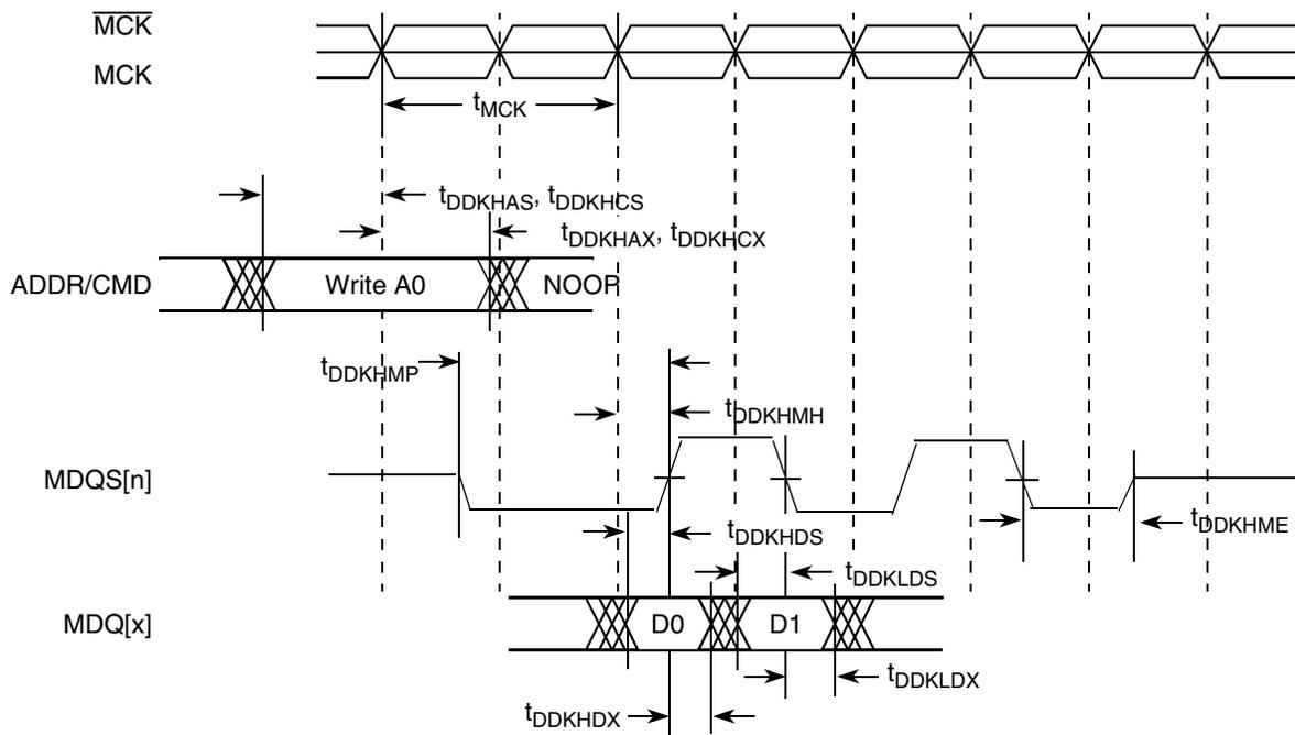
Figure 11. DDR3 and DDR3L Output Timing Diagram
