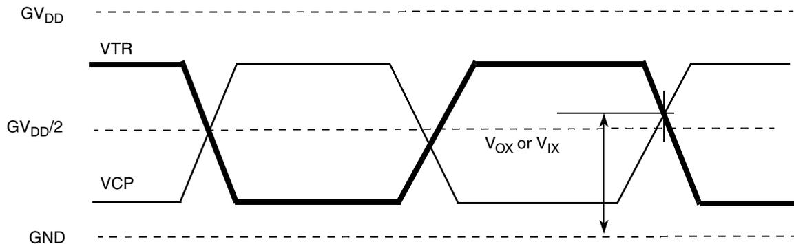
Figure 13. DDR3 and DDR3L SDRAM Differential Timing Specifications
