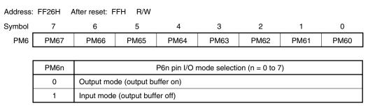
Figure 18-10. Format of Port Mode Register 6 (PM6)
