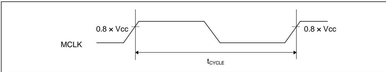
External Bus Signal I/O characteristics
