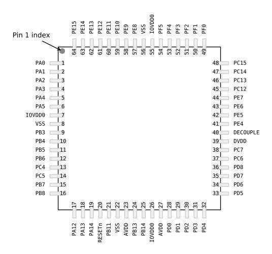
Figure 5.4. EFM32TG11B3xx in QFP64 Device Pinout
