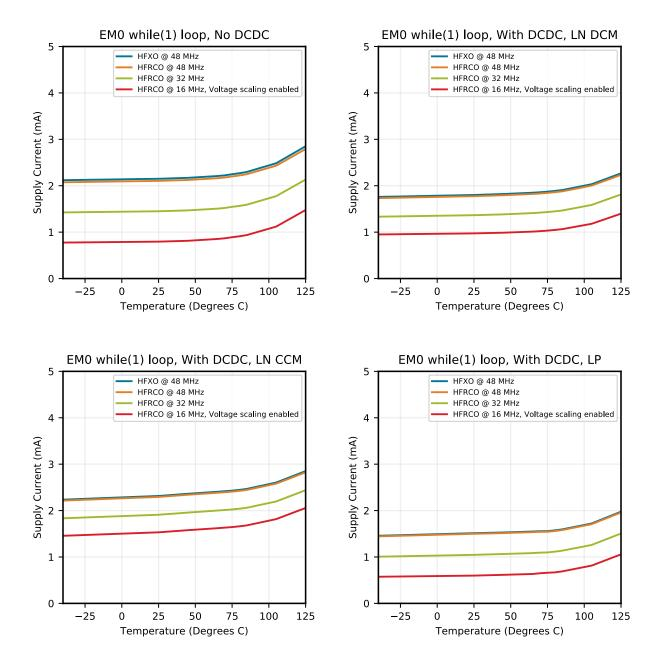
Figure 4.3. EM0 Active Mode Typical Supply Current vs. Temperature
