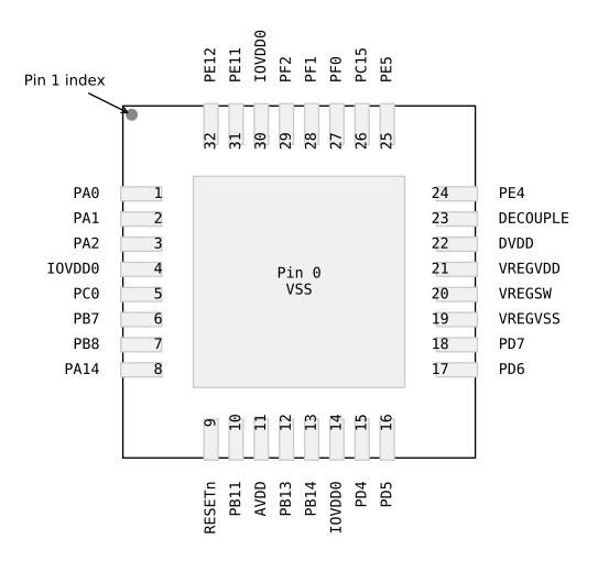
Figure 5.12. EFM32TG11B5xx in QFN32 Device Pinout
