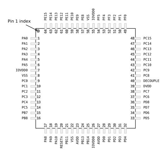
Figure 5.5. EFM32TG11B1xx in QFP64 Device Pinout
