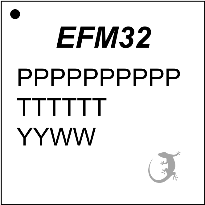
Figure 8.3. TQFP64 Package Marking
