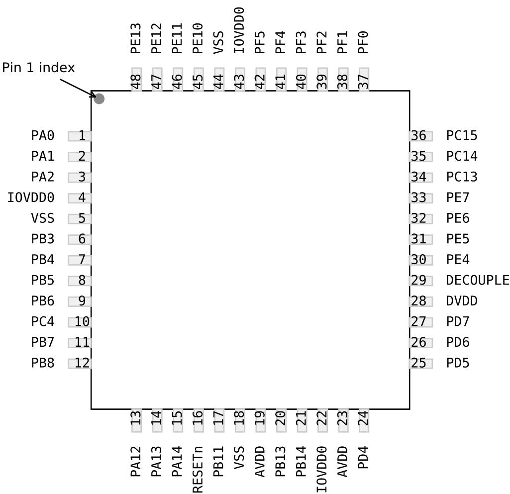
Figure 5.10. EFM32TG11B3xx in QFP48 Device Pinout
