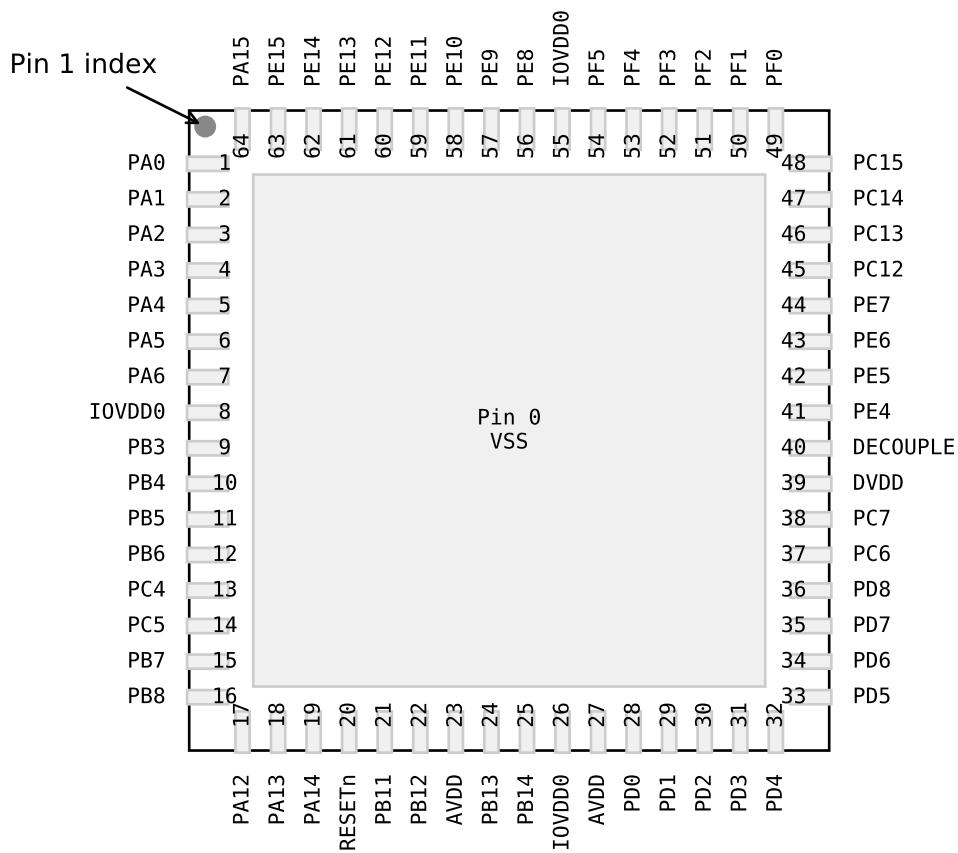
**Figure 5.7. EFM32TG11B3xx in QFN64 Device Pinout**
