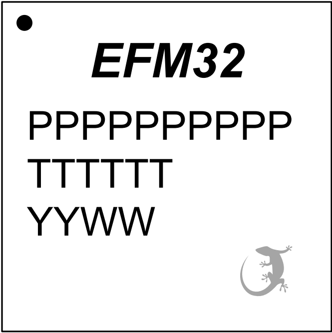
Figure 6.3. TQFP80 Package Marking
