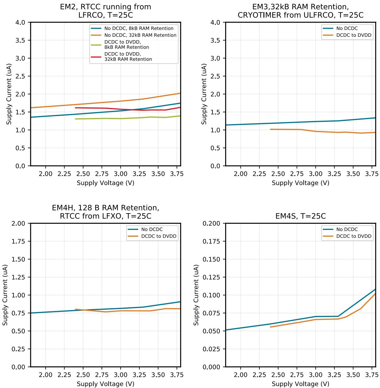
**Figure 4.7. EM2, EM3, EM4H and EM4S Typical Supply Current vs. Supply**
