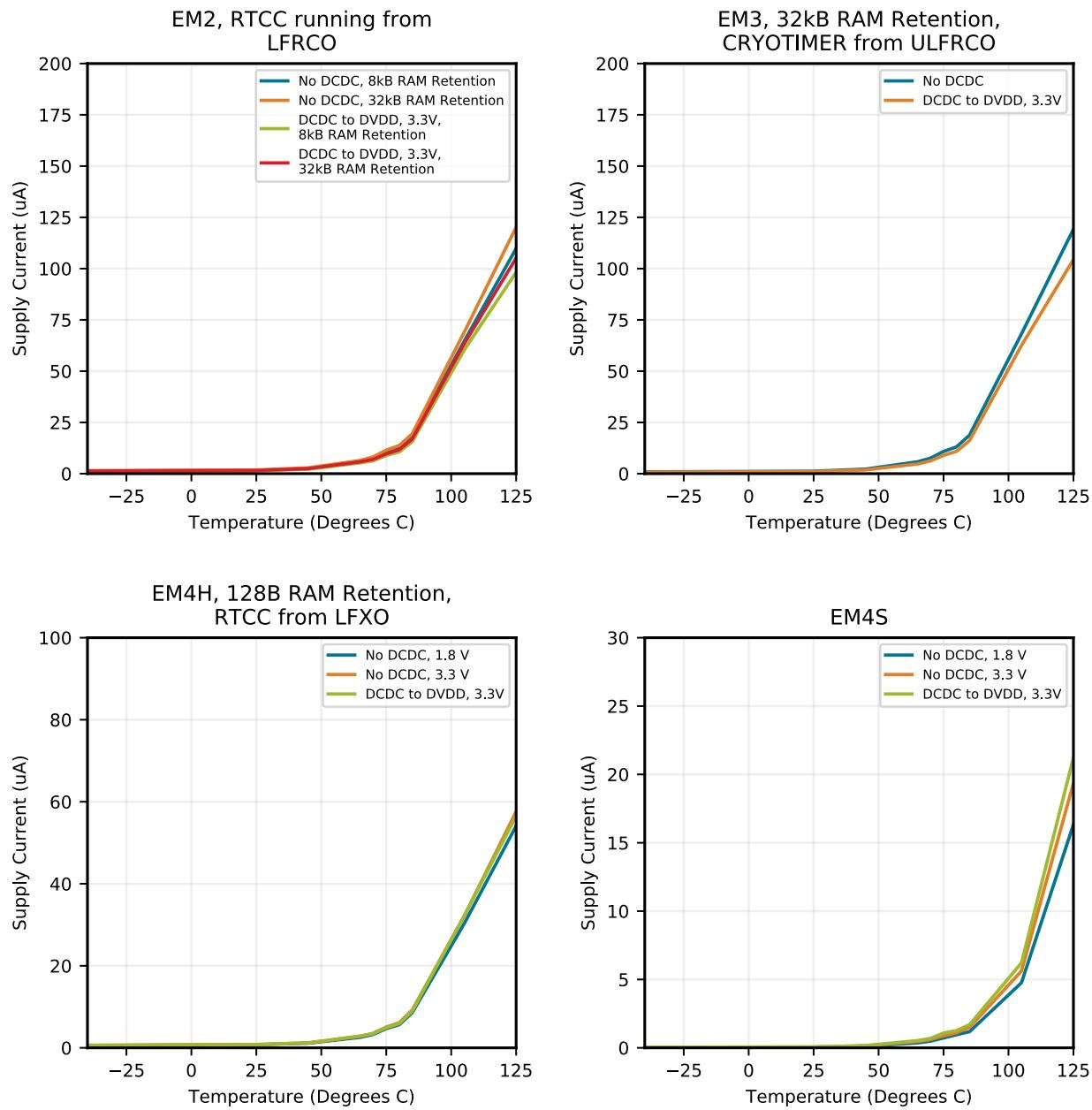
**Figure 4.5. EM2, EM3, EM4H and EM4S Typical Supply Current vs. Temperature**
