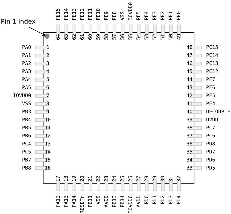
**Figure 5.4. EFM32TG11B3xx in QFP64 Device Pinout**
