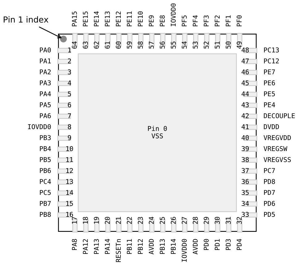
Figure 5.6. EFM32TG11B5xx in QFN64 Device Pinout
