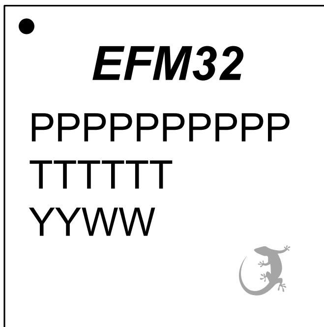
Figure 10.3. TQFP48 Package Marking
