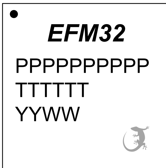
Figure 8.3. TQFP64 Package Marking
