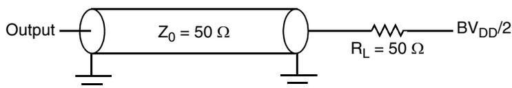
**Figure 56. Enhanced Local Bus AC Test Load**
