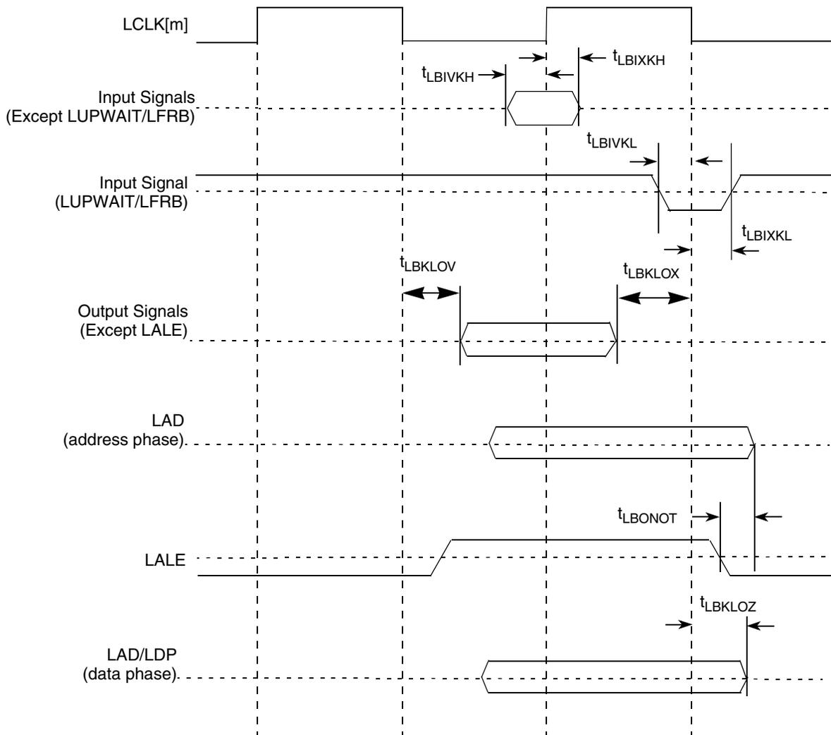
**Figure 59. Enhanced Local Bus Signals (PLL Bypass Mode)**
