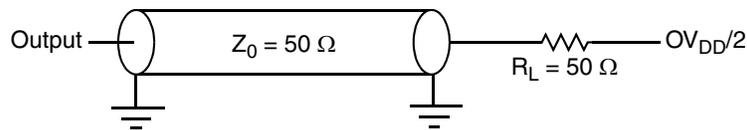
**Figure 52. AC Test Load for the JTAG Interface**
