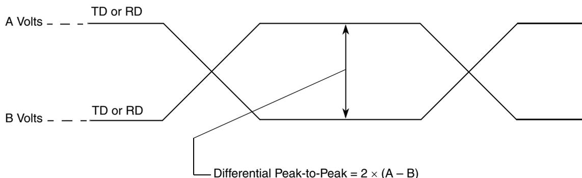
**Figure 47. Differential Peak-Peak Voltage of Transmitter or Receiver**
